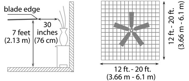
This fan can be mounted with a **downrod** on a regular (no-slope) or vaulted ceiling. The hanging length can be extended by purchasing a longer downrod (0.5 in /1.27 cm diameter). Other installation, such as **flushmount**, is *not* available for this fan.
