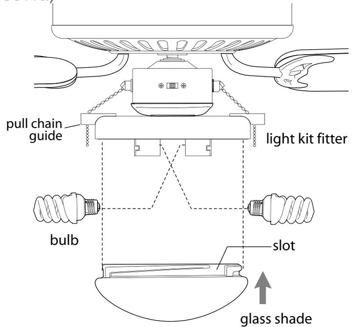
**If you wish to use the fan WITHOUT the light kit,** remove the hex nut and lock washer from the threaded rod at the top of the light kit fitter. Unscrew the switch housing cap to remove it from the light kit fitter and then gently feed the **BLUE (or BLACK)** and **WHITE** wires (one by one) from the light kit fitter through the hole in the middle of the switch housing cap.
